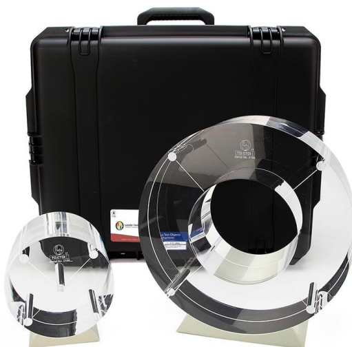
Fig. 5.3. Fantoma standarde CTDI (materiali PMMA)
