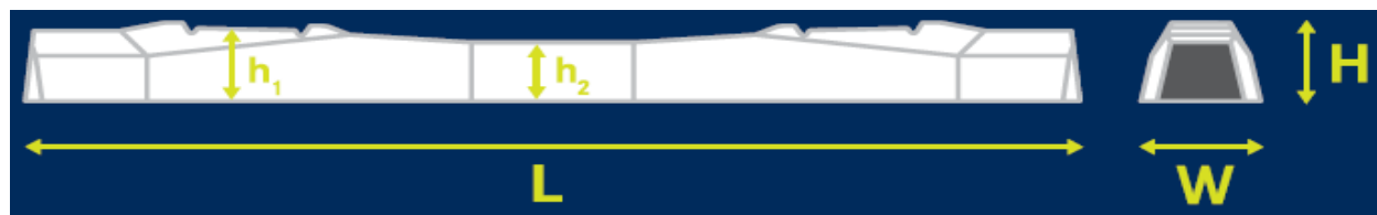
Figura 38: Traversa betony sipas standardit European
