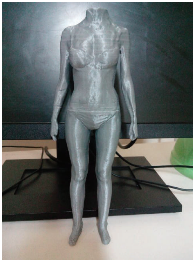
Figura 59. Modeli 3D i trupit i printuar me printerin “Orcabot XXL”.
